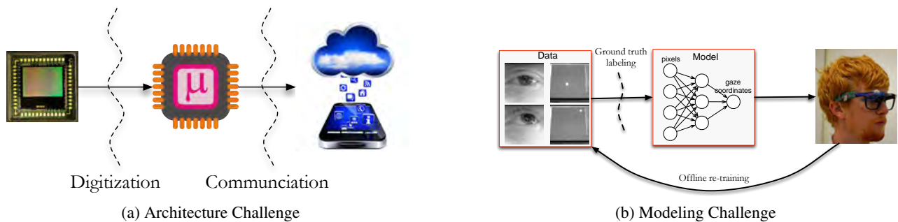
Figure 1: Design challenges. (left) Two major challenges in system design are the power consumed for digitizing pixels from the camera and the power consumed for high-rate communication to a mobile phone. (right) Another major challenge is calibrating the system during online operation without requiring explicit interaction with the user.
